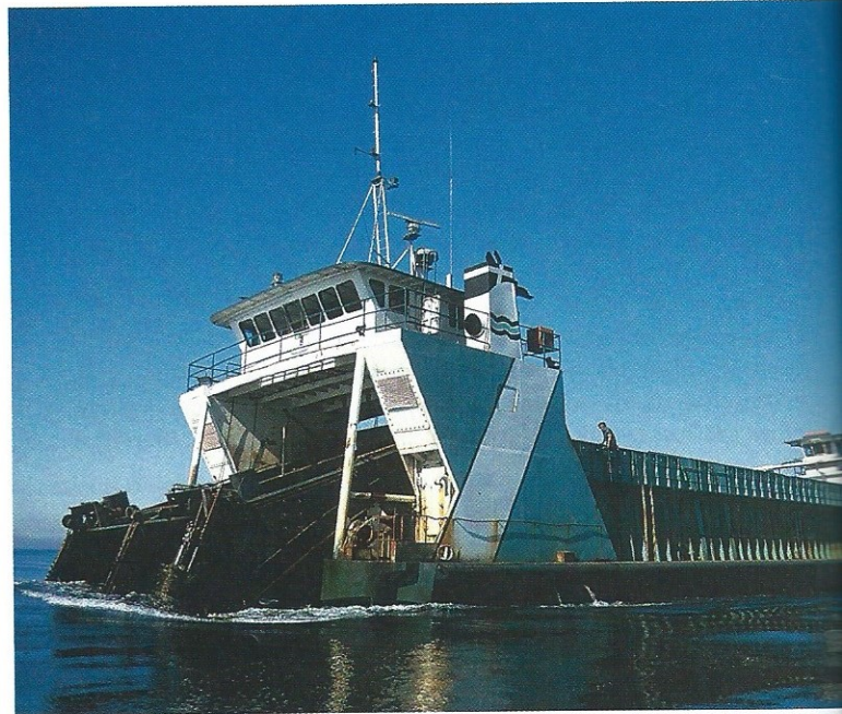
FIGURE 6.12 The Kelstar , a kelp harvester based in San Diego, California. It is 180 ft long and has a capacity of 600 tons.
